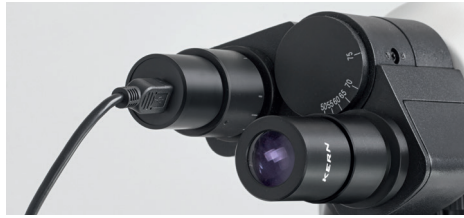
Eyepiece camera fixed into the tube
