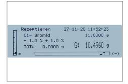
Convenient recipe-weighing with the recipe database, up to 99 recipes can be stored, each with up to 20 recipe ingredients with name and target value
